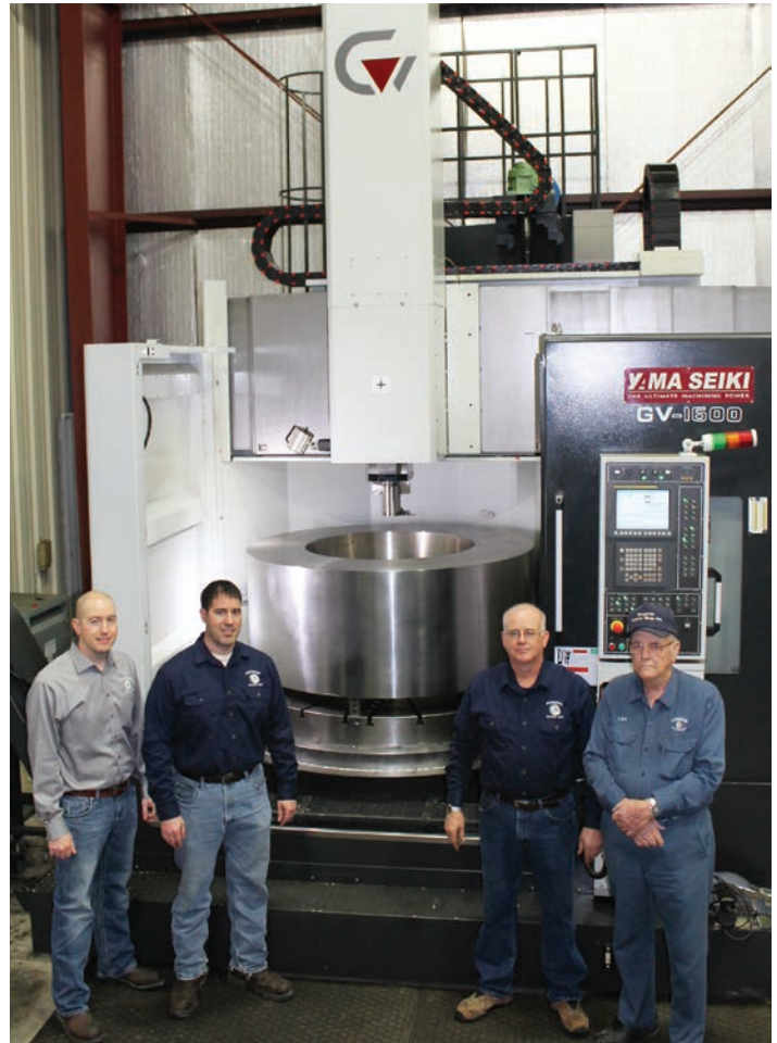
(l-r) Ryan Bergeron, Jarrod Bergeron, Randy Bergeron, Leo Bergeron, all of Bergeron Machine Shop, with the Yama Seiki GV1600 CNC VTL. The part is a 4330 forging, 63" in diameter, 25" tall and weighing 16,000 lbs. They held a 63 surface finish in the I.D. of this part. Forgings of this size require a lot of torque for cutting, which was why a direct gear drive spindle was needed.
