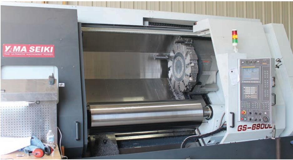
This part, called a mandrel, is 20" O.D. x 65" long 4140 HT. "The Yama Seiki GS6800L CNC horizontal lathe can easily hold +/- .001 tolerance and a 63 finish along the entire length of the part," said Ryan Bergeron, BMS.
